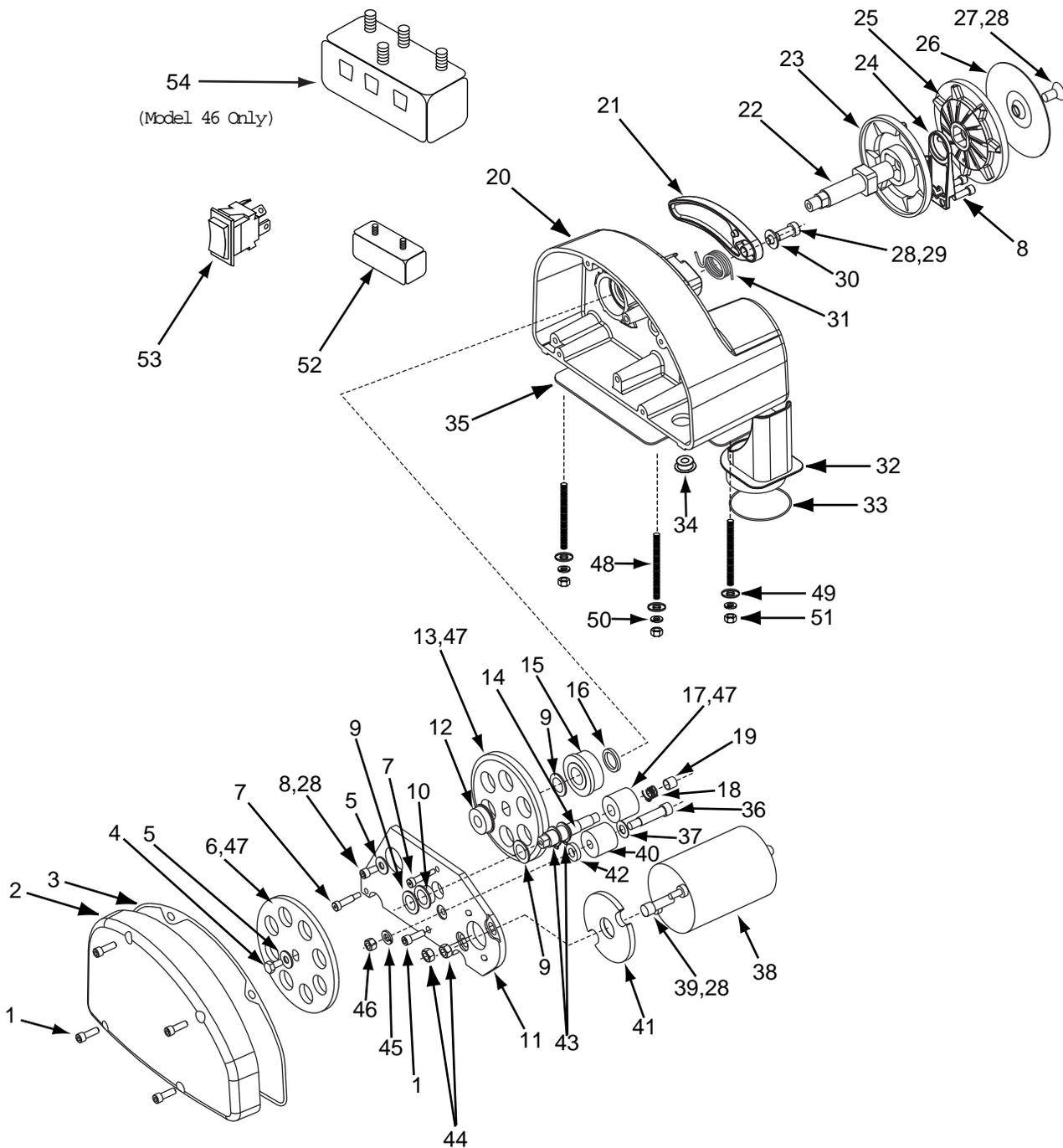
Figure 7 - Replacement Parts Illustration for 31', 36', 41', 46' Class Anchor Winch
